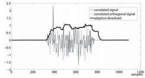
Figure 2. Matlab simulation of symbol synchronization for underwater FSK with a packet consisting of a 15-bit Gold Code sequence followed by 80 bits of data at 15dB SNR
