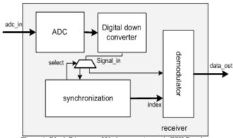
Figure 1. Block Diagram of Underwater Acoustic FSK Receiver
