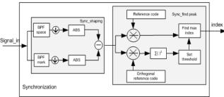
Figure 3. block diagram for symbol synchronization
