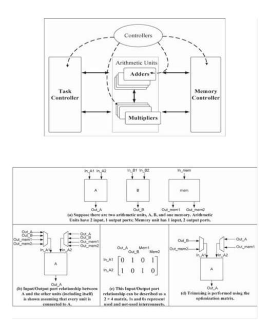
Fig. 7. General-purpose architecture and its datapath.
