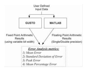
Fig. 9. Performing error analysis using GUSTO.
