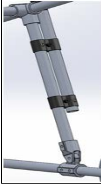
Figure 4-F. Close up view of the rear support with pipe clamps and handle bar
