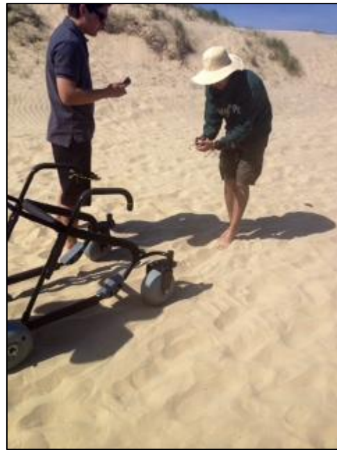
Figure 6-B. Kinetic load testing on sand with digital scale
