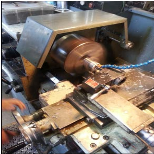
Figure 5-E. Cutting inner diameters of bushing housing using boring tool.
