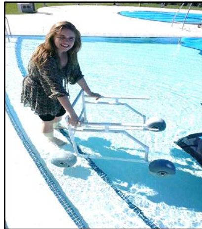
Figure 3-M. Preliminary buoyancy testing of PVC prototype (Jessica)
