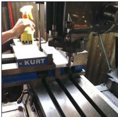
Figure 5-C. Shaping the caster housing pieces on the mill
