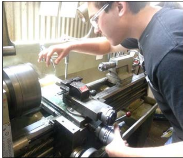
Figure 5-F. Jon manufacturing the nylon bushings.
