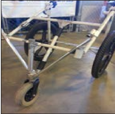
Figure 3-C. Prototype model 2, consisting of two large wheels in front and one rear caster wheel.
