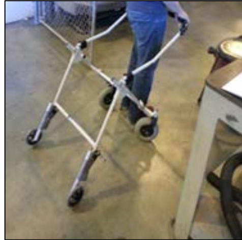
Figure 3-D. Prototype model 3, with two fixed wheels and two free-rotating caster wheels
