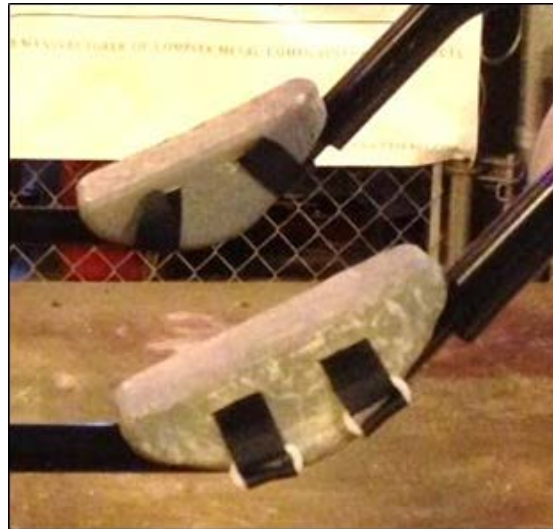
Figure 5-D. Fiberglass coated foam footrests, prior to final paint and hot coat.
