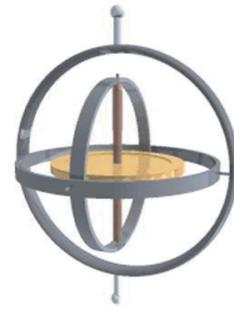
Fig. 1. The two-axis multi-gimbal system
