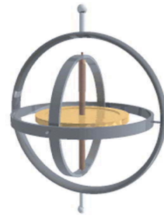
Fig. 1. The two-axis multi-gimbal system
