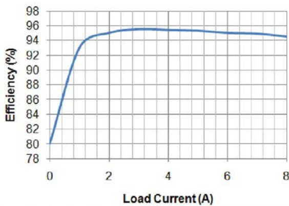
Figure 3. Sample efficiency curve used for individual DC-DC converter characteristics in simulation.
