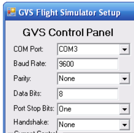
Figure 25 - GVS device default RS-232 connection settings.
