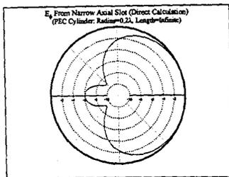
$|E_\theta|$  vs.  $\phi$  Pattern (Direct) for Axial Slot in PEC Cylinder (Radius= $0.2\lambda$ , Length= $\infty$ )
