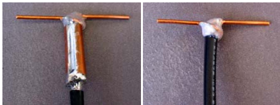
Fig. 9 Dipole with and without Sleeve Balun
