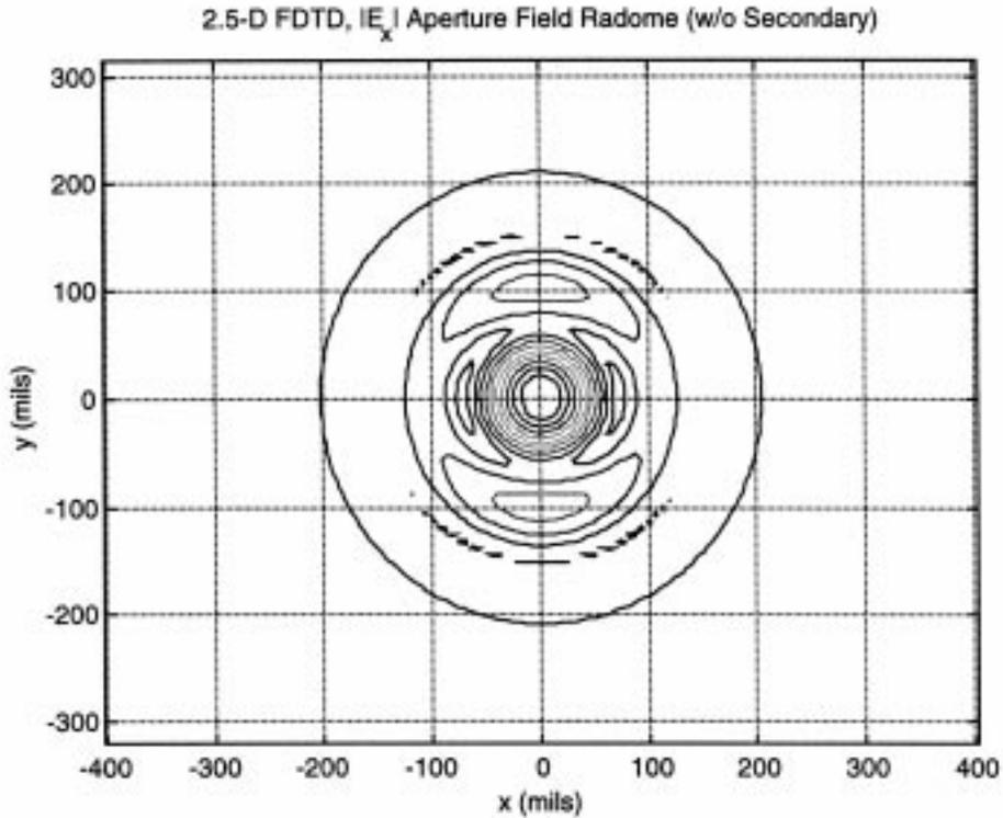
Fig. 10. Aperture field through higher permittivity material ( $\epsilon_r = 8.5$ ).
