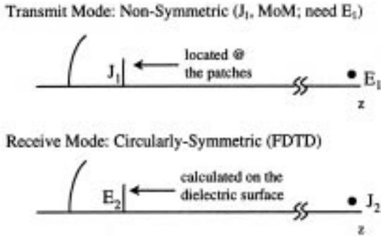
Fig. 3. Application of equivalence and reciprocity theorems to original system.
