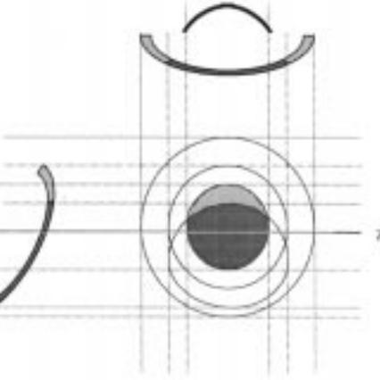
Fig. 7. Tilted radome:  $\theta - \alpha = -90^\circ$ .
