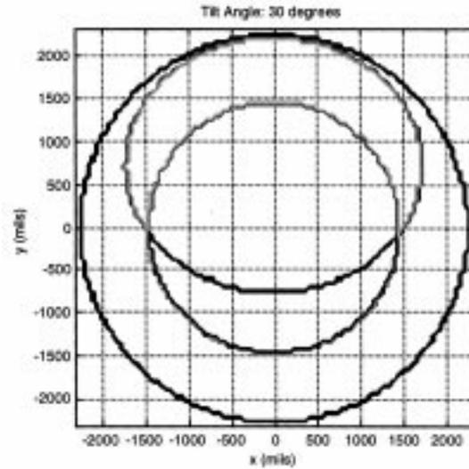
Fig. 12. Elliptical radome pattern projection onto radiating aperture.
