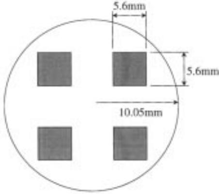
Fig. 2. Microstrip patch antenna geometry.
