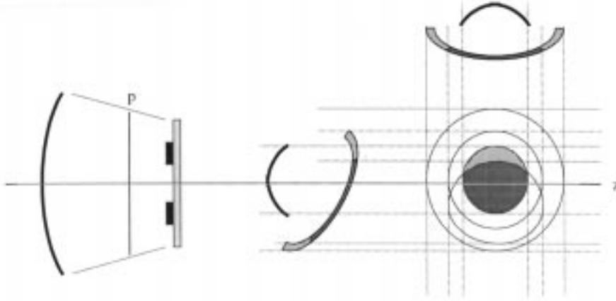
Fig. 5. Tilted radome and projected field distribution.
