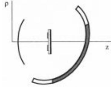
Fig. 4. Reflector antenna system, with tilted radome.
