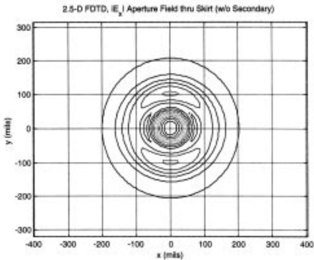
Fig. 11. Aperture field through lower permittivity material ( $\epsilon_r = 4.2$ ).
