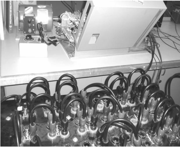
Figure 2. DC Drive (top) is connected to resistor load bank (bottom)
