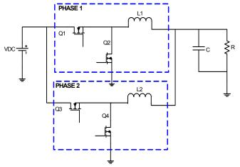
Fig 1. Multiphase synchronous buck topology.
