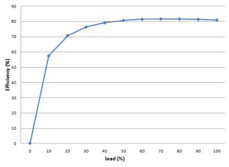
Fig. 8. Efficiency of the proposed converter with load variation
