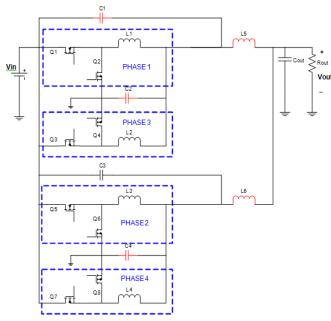
Fig. 2. Proposed multiphase interleaved buck topology
