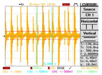
Fig. 6. Output voltage ripple at full load
