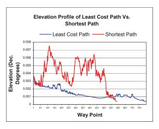
Figure 2. An elevation graph comparing two types of paths between the same source and destination for the terrain shown in Figure 1. Note that the shortest path includes substantial elevation gains, while the least cost caloric path takes a much more level path.
