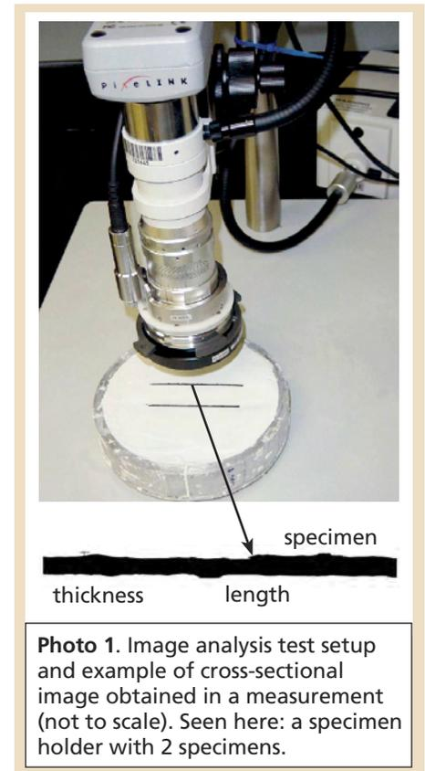
**Photo 1.** Image analysis test setup and example of cross-sectional image obtained in a measurement holder with 2 specimens. (not to scale). Seen here: a specimen holder with 2 specimens.
