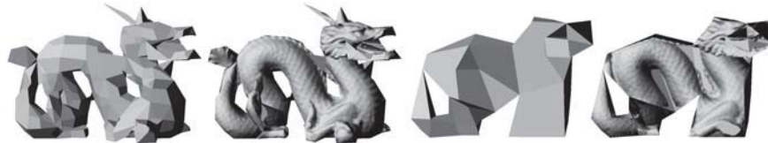
Fig. 6. Left two: flat-shaded and normal mapped dual contour surface (558 quads). Right two: flat-shaded and normal mapped dual contour surface (65 quads).
