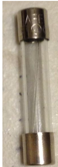
Figure 3-4: Fast-Acting, AGC Fuse; Rated at 8A, 250V
