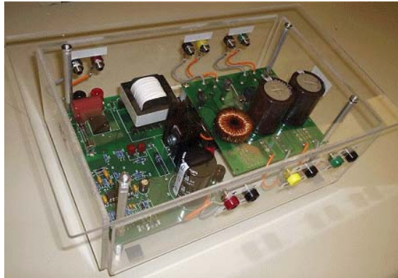
FIGURE 9 Active Power Factor Correction Module
