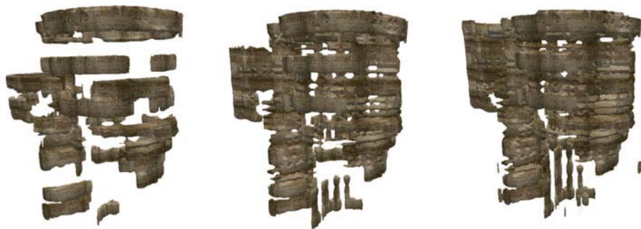
Fig. 5. Three side view images of the Mdina archive, on the right is the archive with no diffusion, then one step, then two. Note that Figure 4 illustrates the final shape of the archive geometric model.
