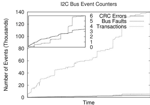
Figure 1. I<sup>2</sup>C bus event data from CP6. Inset in upper left shows only the CRC error and bus fault event counters. Time progresses left-to-right, but not proportionally due to periods of time when no data was downlinked.
