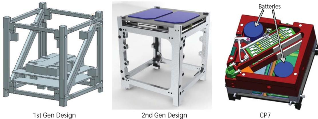
Figure 2. CAD Renderings of different PolySat satellites. The CP7 rendering illustrates how mission-specific batteries were utilized in the payload bay.
