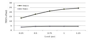
Figure 7. Trend of voltage distortion in varying operation speed and loading level of ASD
