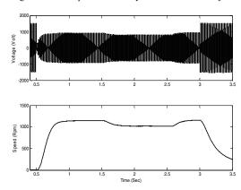
Figure 9. ASD Input voltage and motor speed when irradiance is adjusted as Fig. 8.
