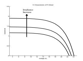
Figure 1. Dependence of V- I characteristic of a PV module due to irradiance variation
