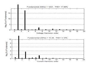
Figure 6. Grid distortion during single phase ASD operation
