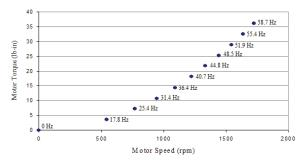
Figure 2. Torque and Frequency Values Associated with Measurements
