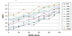
Figure 9. THD<sub>V</sub> vs. M3/M4 Load at Location B
