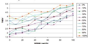
Figure 10. THD<sub>V</sub> vs. M3/M4 Load at Location C
