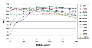
Figure 12. THD<sub>I</sub> vs. M3/M4 Load at Location A
