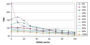
Figure 13. THD<sub>I</sub> vs. M3/M4 Load at Location B
