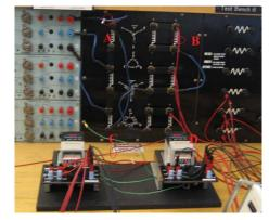
Figure 5. Adjustable speed drives in the laboratory setup
