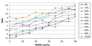
Figure 11. THD<sub>V</sub> vs. M3/M4 Load at Location D
