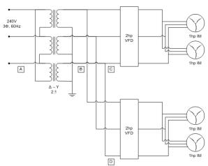
Figure 1. Diagram of system configuration
