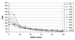
Figure 14. THD<sub>I</sub> vs. M3/M4 Load at Location C
