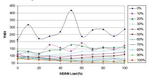
Figure 15. THD<sub>I</sub> vs. M3/M4 Load at Location D
