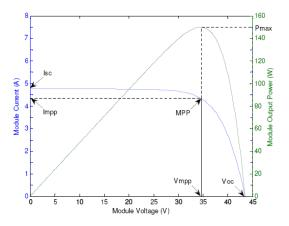
Figure 7. I-V and P-V relationships of PV module
