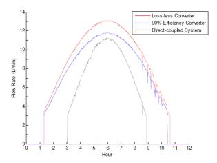
Figure 15. Flow rates of PV water pumps
