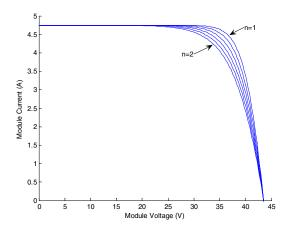
Figure 3. Effect of diode ideally factors
