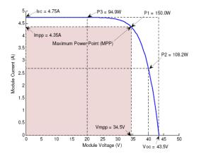
Figure 6. Simulated I-V curve of PV module
