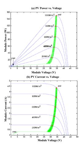
Figure 14. MPPT simulations with the DC pump motor load (20 to 1000 W/m2,  $25^{\circ}C$ )
