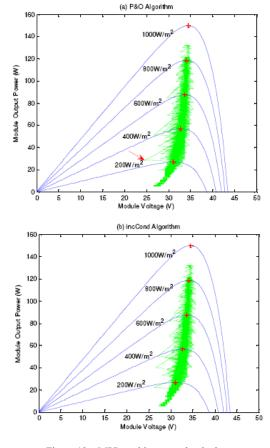
Figure 12. MPP tracking on a cloudy day
