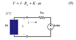
Figure 8. Electrical model of permanent magnet DC motor
