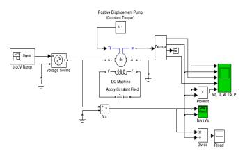
Figure 13. Simulink model for DC Motor
