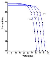
Figure 5. I-V curves for various temperatures
