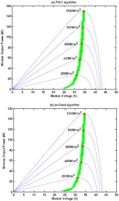
Figure 11. MPP tracking on a sunny day
