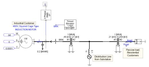
Figure 5. Power distribution system model with shunt capacitor
