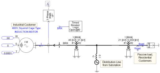
Figure 2. Basic power distribution system model
