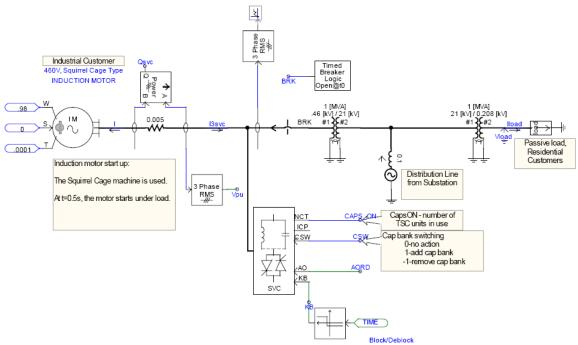
Figure 6. Power distribution system model with SVC
