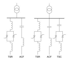
Figure 1. Typical SVC configuration
