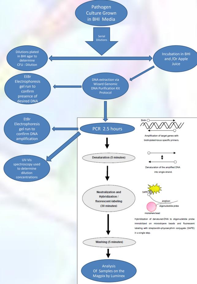
Figure 1: Schematic of the overall testing process.
