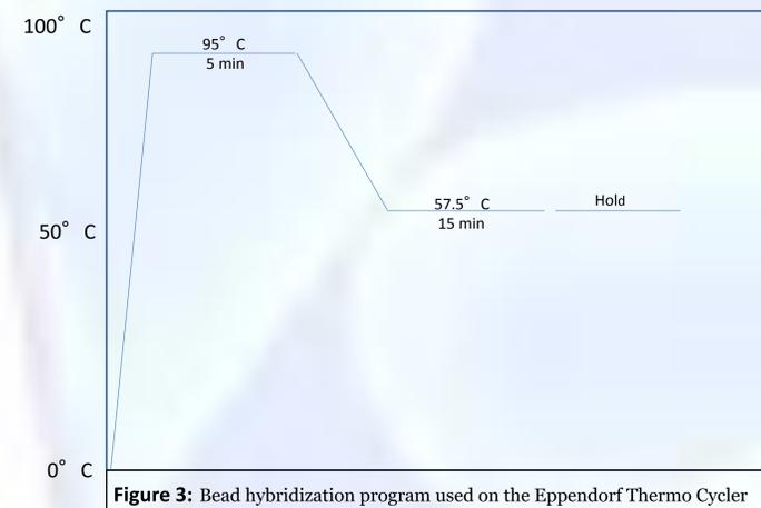
Figure 3: Bead hybridization program used on the Eppendorf Thermo Cycler
