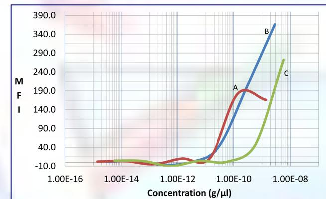
Figure 4: Median Fluorescence Intensity (MFI) is the unit of measure of the Magpix by Luminex apparatus. (A) *Listeria monocytogenes* (ATCC7644) (B) *Salmonella enterica* Typhi (ATCC14028) (C) *Escherichia coli* (ATCC43889)
