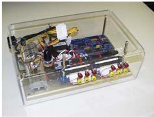
Figure 7. Enerpro's Thyristor Firing board
