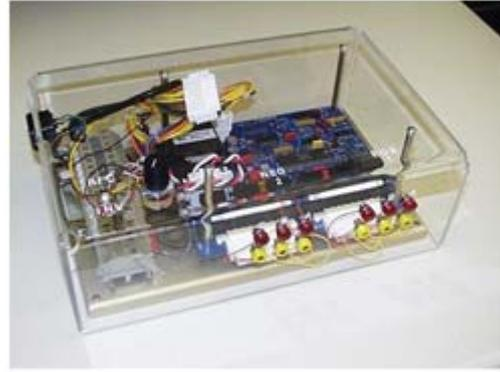
Figure 7. Enerpro's Thyristor Firing board
