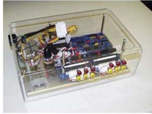
Figure 7. Enerpro's Thyristor Firing board
