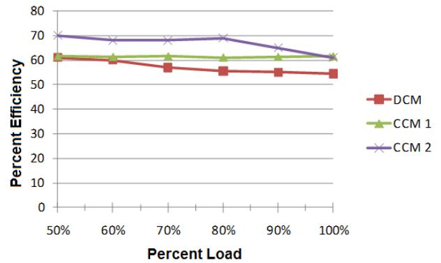
Figure 11. Percent efficiency as a function of load
