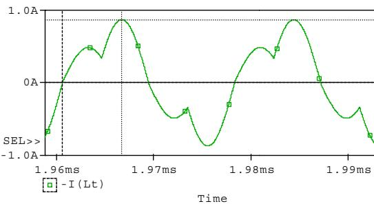
Figure 4. CCM 1 inductor current waveform
