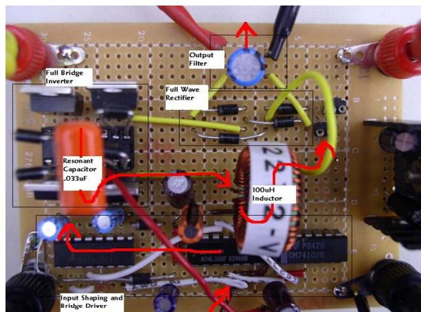
Figure 7. SLR converter circuit
