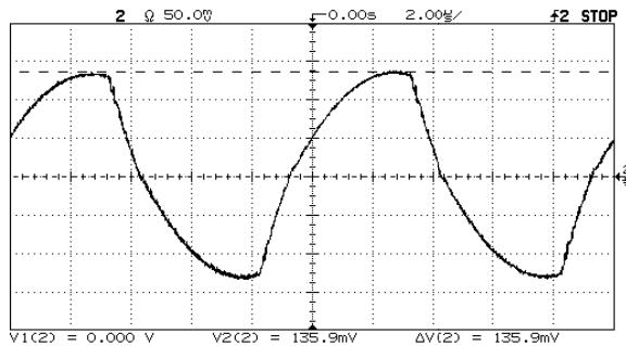
Figure 10. CCM 2 inductor current waveform
