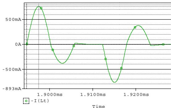
Figure 3. DCM inductor current waveform
