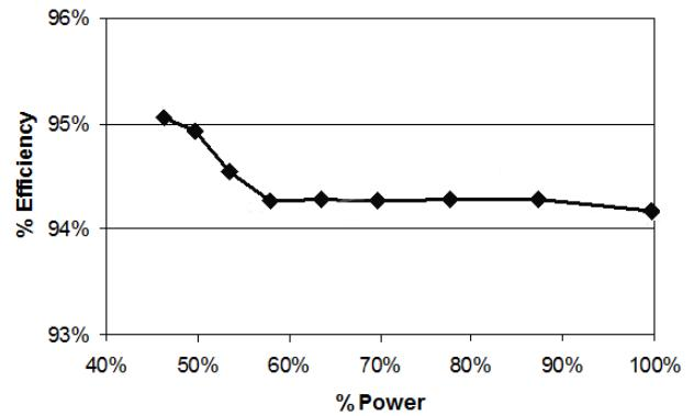
Figure 6. Efficiency of SLR in CCM 1 mode
