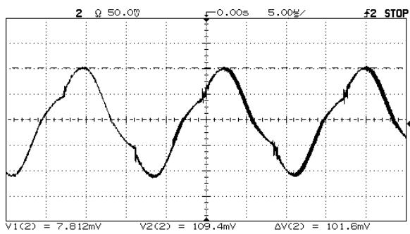
Figure 9. CCM 1 inductor current waveform
