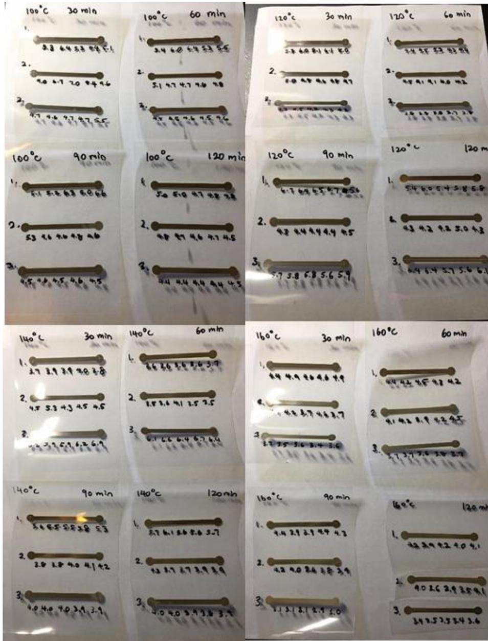
Figure 4. 16 printed sample films with each sheet for one set of curing conditions.
