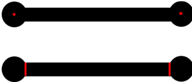
Figure 12. Measuring resistance using one point on each end (top) measuring across the width (bottom).
