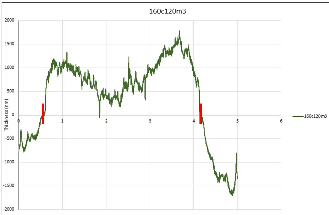
Figure 6. Example of a profilometer graph generated. For the first model, the thicknesses for the ink traces were calculated by averaging the data points from where the ink trace begins and ends, represented by the two red lines.
