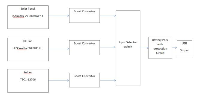
Figure 2-1 Block Diagram of design
