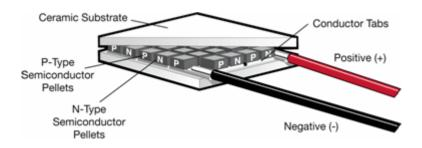
Figure 3-3 Basic structure of Peltier cells
