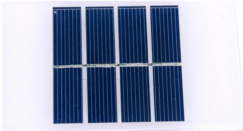
Figure 3-1 Solmaxx 2V solar panel
