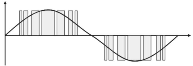
Fig. 6. Pulse width modulation signal compared to sinusoidal
