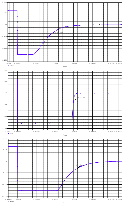
Figure 3. Simulated reverse recovery characteristics for schottky (top), pn (middle), and SBR (bottom).
