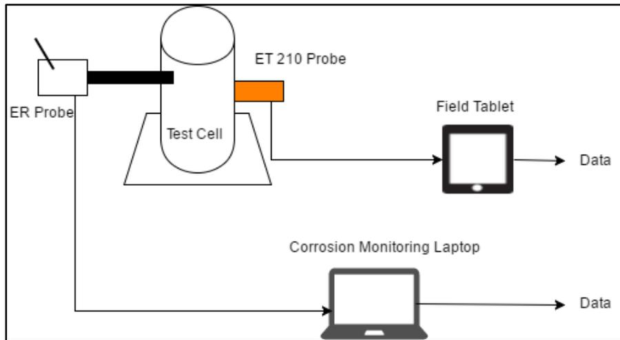
Figure 5. Schematic of static system for the testing of corrosion monitoring.
