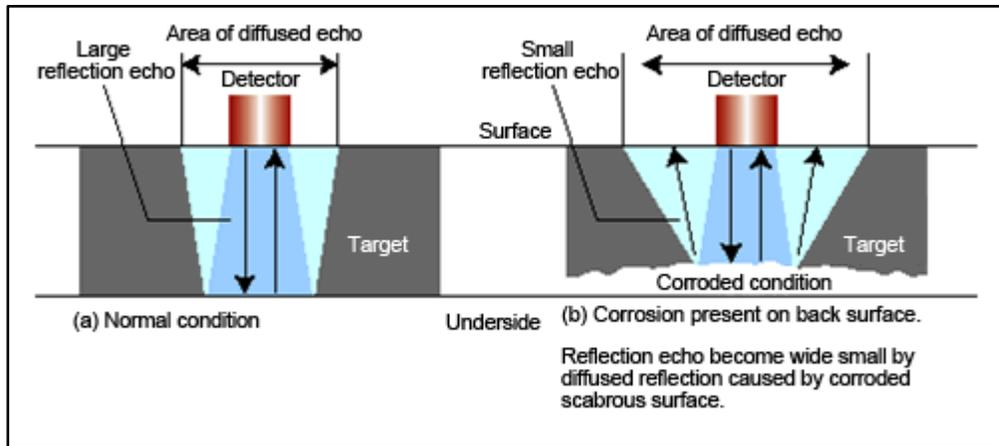
Figure 3. How a simple ultrasonic measuring devices records pipeline thickness.
