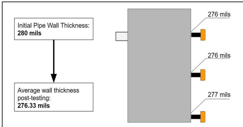
Figure 7. Depiction of additional wall thickness measurements using the ET-210 WiHART Sensor.
