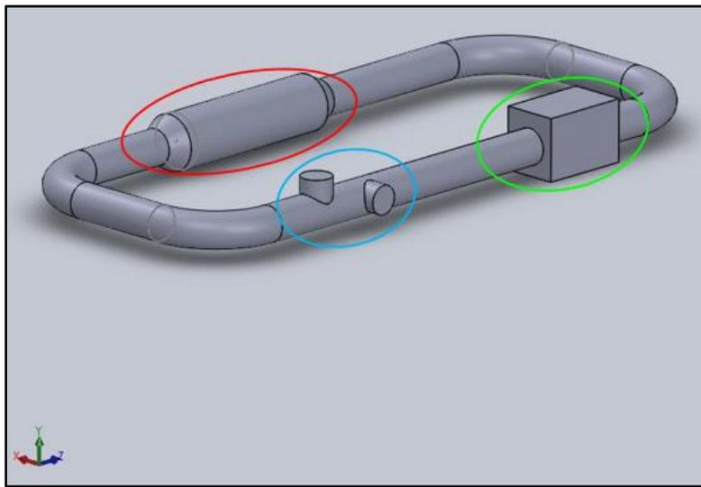
Figure 4. Dynamic low flow system considered to replicate a corrosive environment found in fuel processing systems (Test section = red circle, access valves = blue circle, pump = green circle).
