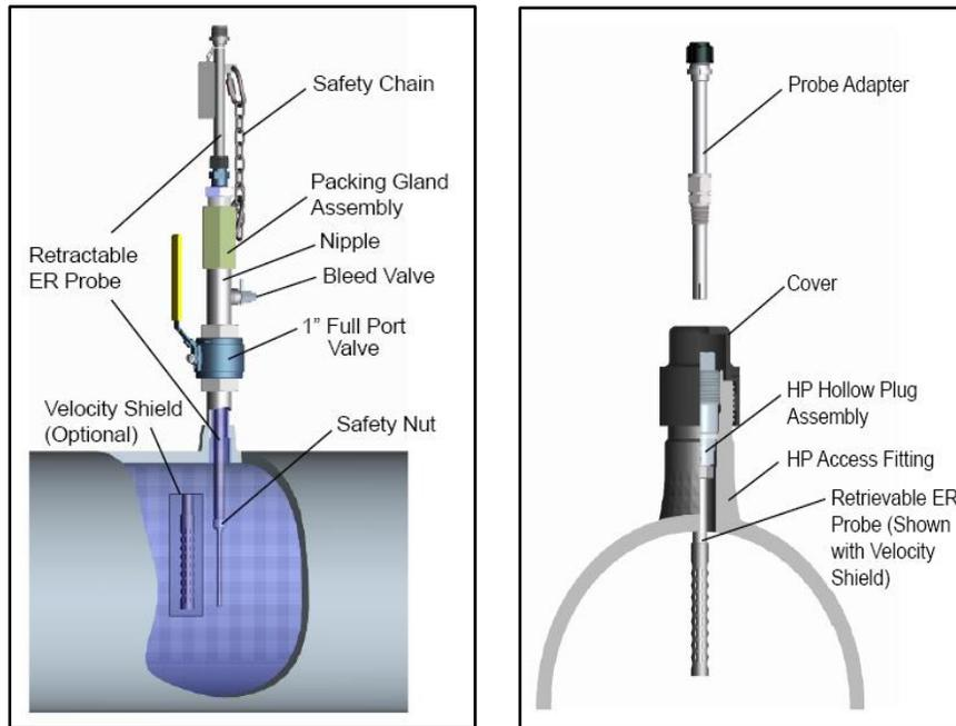
Figure 1. Typical designs for a retractable (left) and retrievable (right) corrosion monitoring ER probe variant. [<http://www.alspi.com/erintro.htm>]
