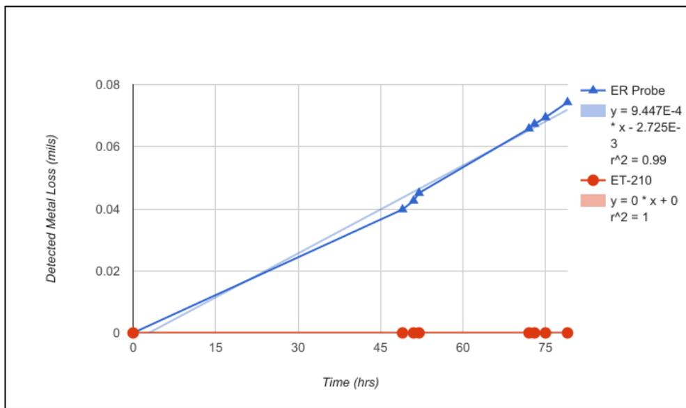
Figure 6. Data showing metal loss over time measured by the two devices.
