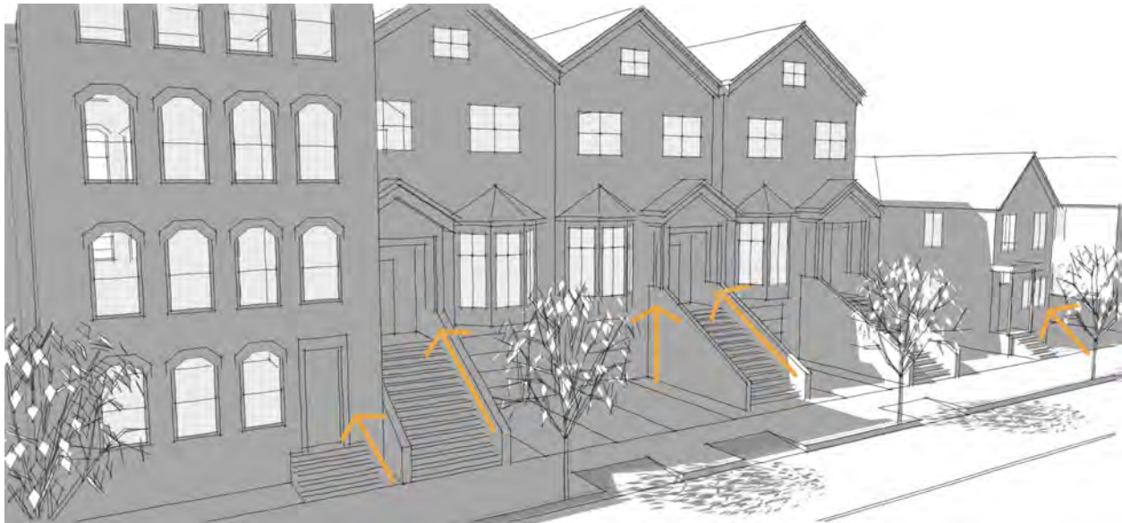
Figure 4.2 – 1: Raising residences above street-level separates the private realm from the shared public space.
