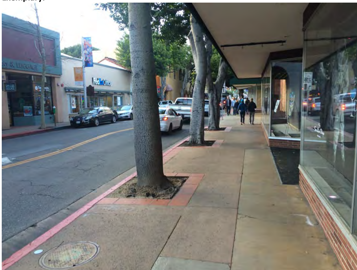
Figure 4.3 – 4: The number of interruptions on a sidewalk should be limited to make the main corridor as contiguous as possible.
