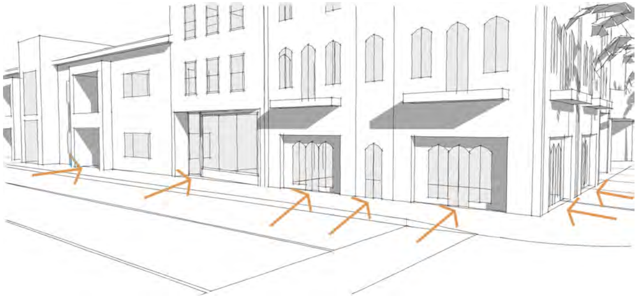
Figure 4.2 – 8: Buildings and their subsequent uses should be as accessible to as many users as possible. Increasing the number of entrances does just that. Accessibility can often deter people from visiting certain locations; better accessibility removes that hindrance.
