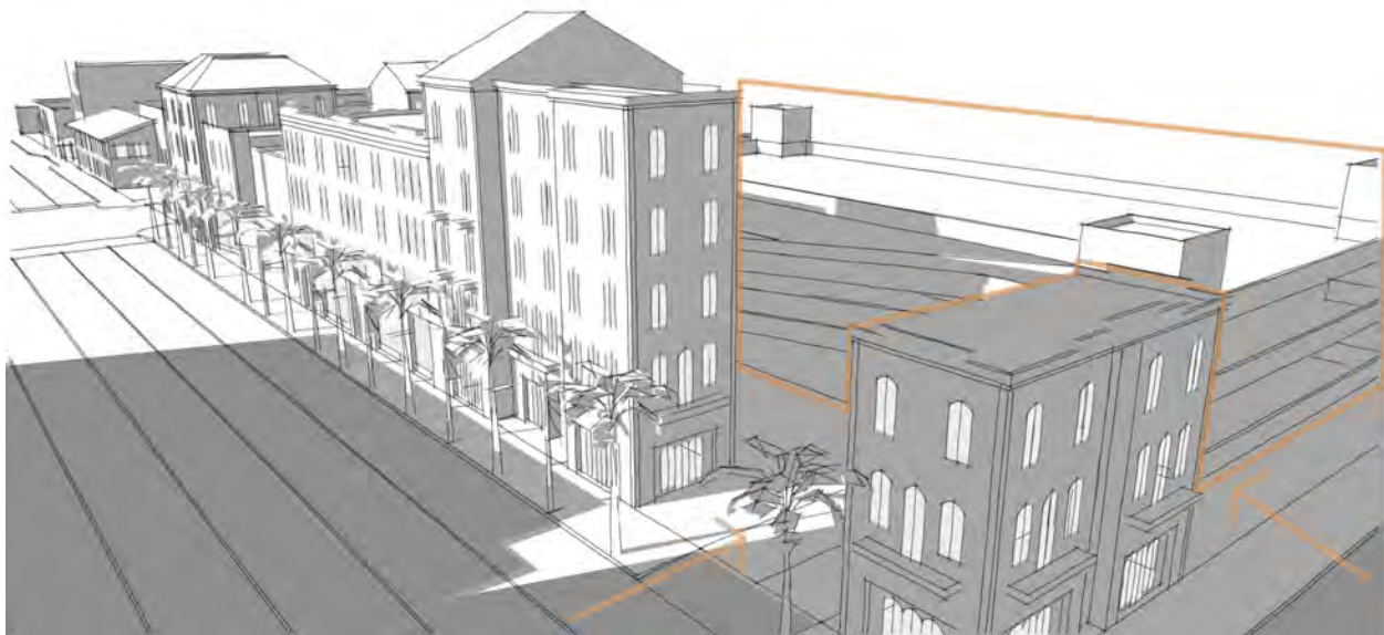
Figure 4.3 – 1: Not all parking can or should be eliminated, but it can be rearranged away from the corridor to mitigate its negative impacts on the streetscape.
