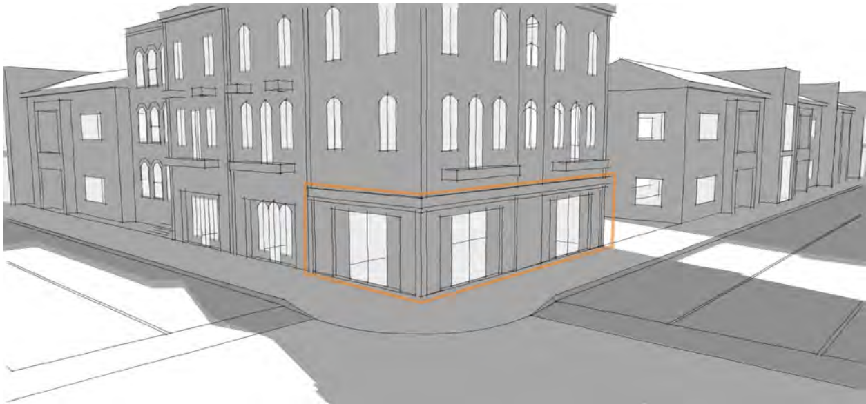
Figure 4.2 – 6: Using various articulations, cornices, columns, and door and window treatments, the ground-floor use can be differentiated from the upper floors. This draws attention to the first-floor use, and in coordination with adjacent buildings makes the corridor more cohesive and readable.
