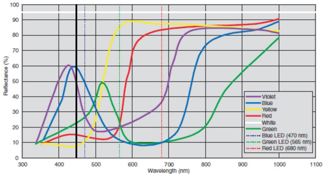
**Figure 4** – Reflectance values from an OMRON photoelectric sensor with black vertical line highlighting reflectance values corresponding to  $\lambda = 450\text{nm}$
