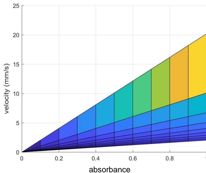
**Figure 6** – Graph depicting the direct relationship between cut velocity and absorbance.
