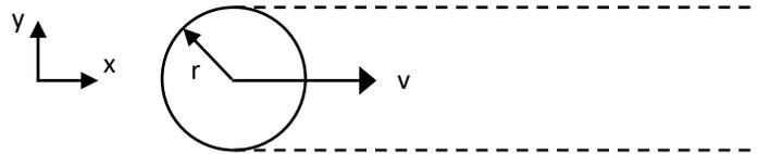
**Figure 3** – Top view of circular cross-section of laser beam predicted cut area resulting from motion of laser along x-direction.
