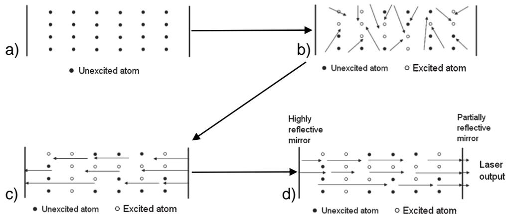
**Figure 1** – Schematic of light amplification stages: (a) initial unexcited state (laser off), (b) optical pumping resulting in an excited state, (c) stimulated emission, and (d) amplification of light.
