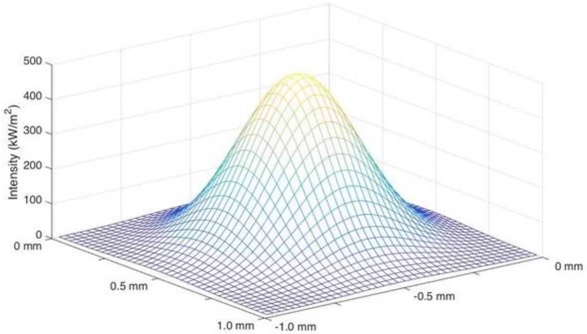
**Figure 2** – Laser in Transverse Electromagnetic Mode ( $TEM_{00}$ ) showing a Gaussian spatial distribution. By assuming the beam has a circular cross-section, it will move with a defined velocity along a central line in the x-direction, as shown in Figure 3.
