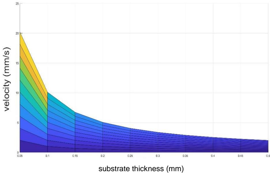
**Figure 7** – Graph depicting the inverse relationship between cut velocity and substrate thickness.
