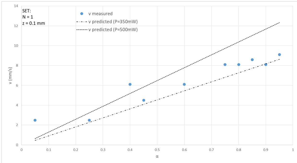
**Figure 9** – Dashed lines depict upper and lower bounds of predicted cut velocity with dots representing the measured cut velocity for optimal cuts.
