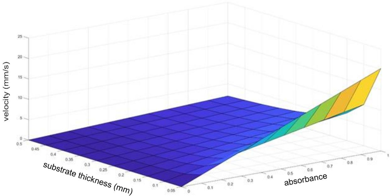
**Figure 5** – Surface plot of thickness and absorbance effects on cut velocity given 1 laser pass.
