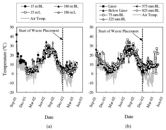
Figure 2. Bottom liner temperatures in Cell D.
