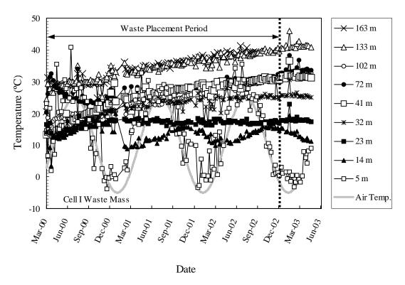
Figure 4. Waste mass temperatures in Cell I.
