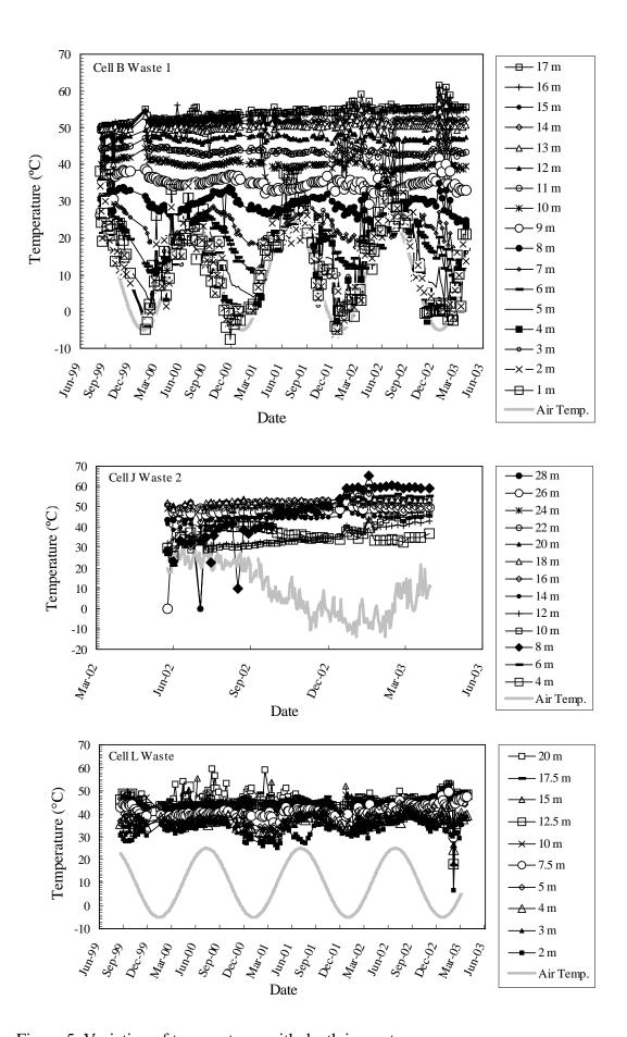
Figure 5. Variation of temperatures with depth in waste.
