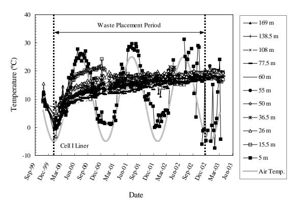
Figure 3. Bottom liner temperatures in Cells J and I.
