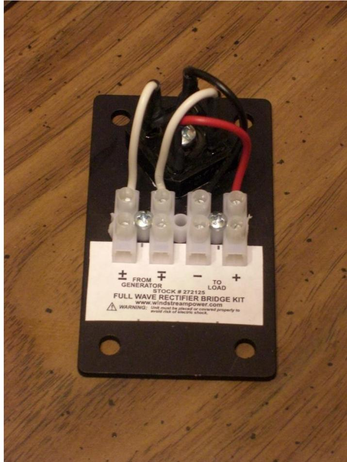
**Figure 5 - Full-Wave Bridge Rectifier**
