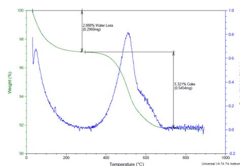
Figure 4. Weight loss (green) and weight loss derivative (blue) of a stage 2 sample. Initial mass loss represents water. Second mass loss represents coke and occurs in two distinct events indicated in the asymmetrical features of derivative curve.
