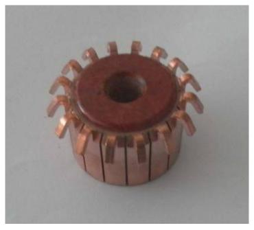
Figure 8: Commutator with hooks for connections [2]
