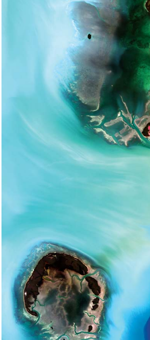
ABOVE AND PRECEDING THREE SPREADS: Three bands (RGB= 666, 547, 439 nm) from a March 23, 1996 Air borne Visible/Infrared Imaging Spectrometer (AVIRIS) image taken over the Florida Keys from an ER-2 aircraft at 20 km above ground. The top of the image is near the eastern end of the Keys; the bottom of the image is near the western end. The rough heading is 260 degrees (clockwise from north) top to bottom (i.e., just south of west). AVIRIS is an optical sensor that delivers calibrated images of upwelling spectral radiance in 224 contiguous spectral channels (bands) with wavelengths from 400 to 2500 nanometers. Note that this image is not atmospherically corrected. It is \pi \times \text{radiance} / [\text{mean\_solar\_ir\_radiance\_at\_the\_top\_of\_the\_atmosphere} \times \cos(\text{solar\_zenith\_angle})] . Original data courtesy of NASA/JPL. Caption courtesy of Marcos Montes of Naval Research Laboratory, Washington D.C.
