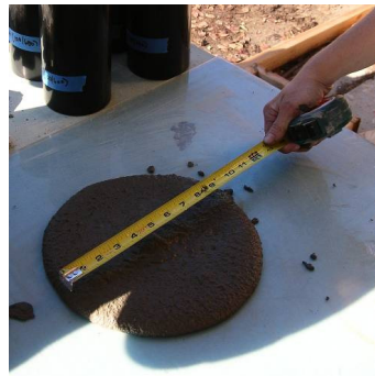
FIG. 2. Testing for Flow
