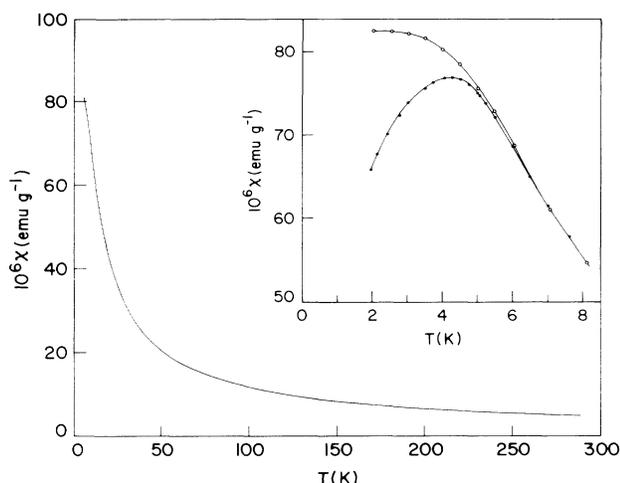
FIG. 1. Temperature dependence of magnetic susceptibility of the quasicrystal  $i\text{-Al}_{74}\text{Mn}_{15}\text{Fe}_5\text{Si}_6$ . Inset: Expanded plot of the low-temperature susceptibility for a sample initially cooled in zero field (filled circles) and one initially cooled in a magnetic field of 50 Oe (open circles).
