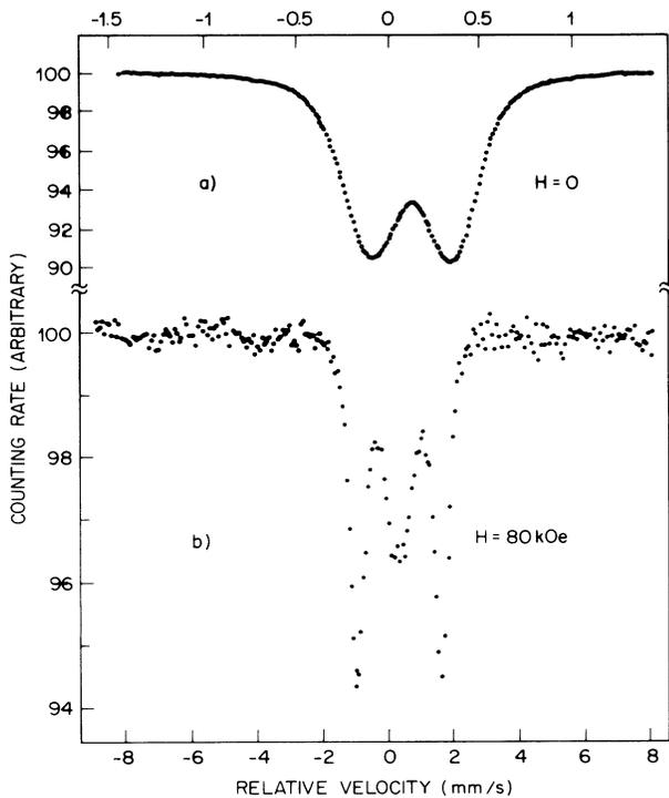
FIG. 2. (a) The  $T=4.2$  K Mössbauer spectrum of quasi-crystalline  $i\text{-Al}_{74}\text{Mn}_{15}\text{Fe}_5\text{Si}_6$  and (b) the  $T=4.2$  K Mössbauer Zeeman spectrum of the same sample in a magnetic field  $H=80$  kOe applied parallel to the direction of  $\gamma$ -ray propagation.
