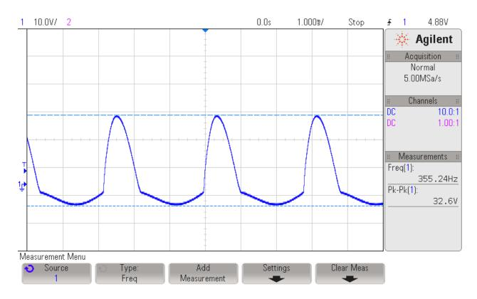
Figure 6: Voltage waveform for dynamo characteristics at gear 4.
