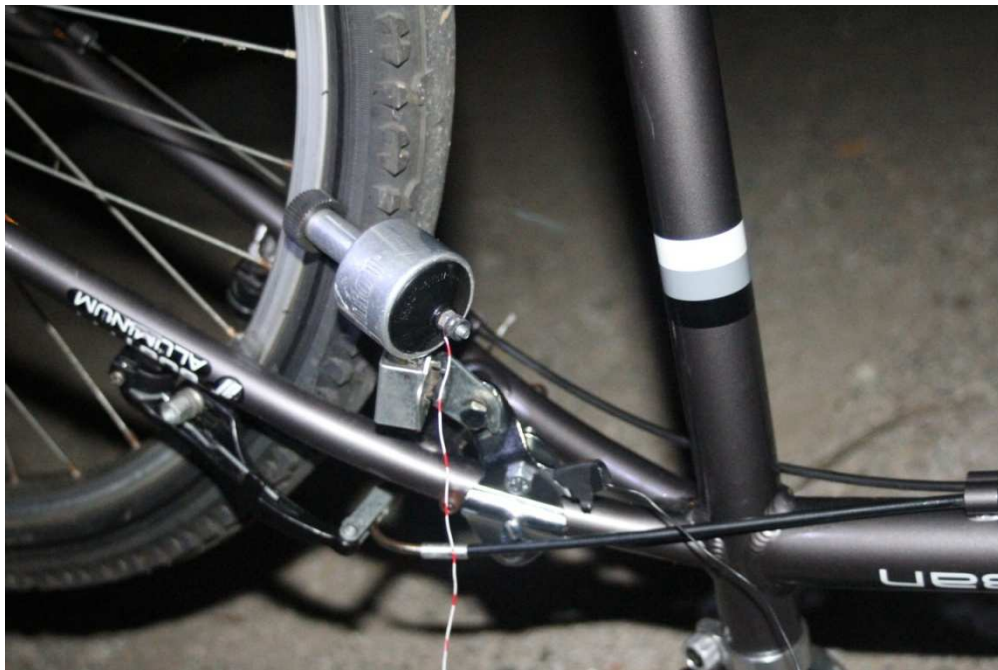
Figure 5: Dynamo mounted to bicycle frame.
