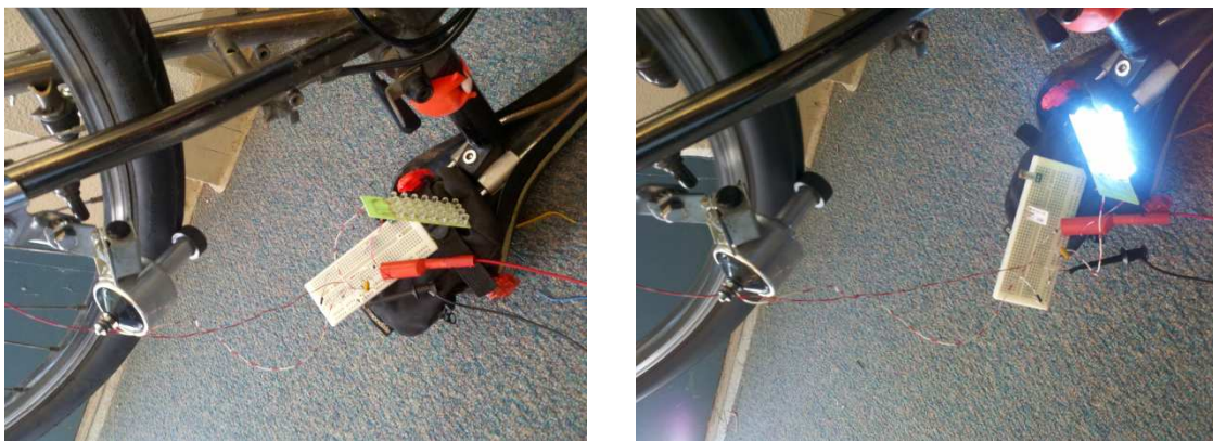
Figure 10: Testing circuit with LEDs off (left) and LEDs on (right).
