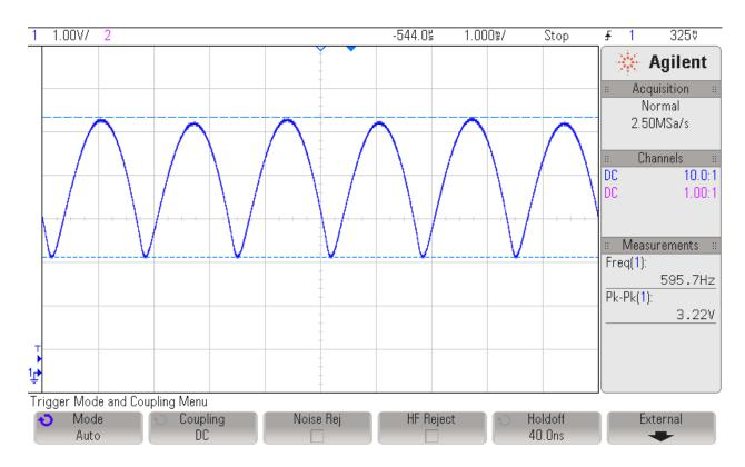
Figure 8: Voltage waveform for full wave rectifier with capacitor at gear 4.
