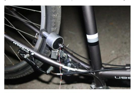
Figure 5: Dynamo mounted to bicycle frame.
