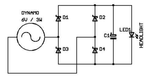
Figure 2: Basic LED headlight with capacitor in parallel.
