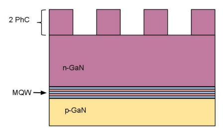
Figure 6 GaN thin film LED with a photonic crystal grating.
