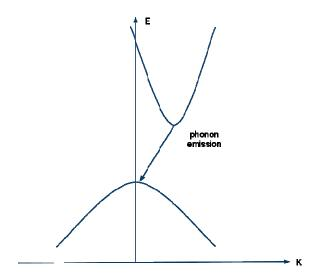
Figure 2 Example of an indirect band gap emitting a phonon Gallium Nitride's variable band gap also makes it extremely useful for light emitting devices. For example, adjusting the composition of  $In_xGa_{1-x}N$  can vary the band gap from 1.9eV to 3.4eV.<sup>4</sup> The equation below shows that the wavelength of light emitted depends indirectly on the energy of the gap.
