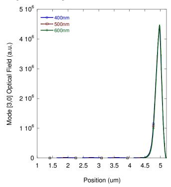
Figure 9 Mode [3,0] optical field vs position for AlGaN thicknesses 400, 500, 600nm
