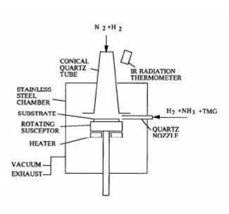
Figure 3 Two flow MOCVD diagram
