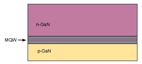
Figure 5 GaN thin film LED without photonic crystal grating.
