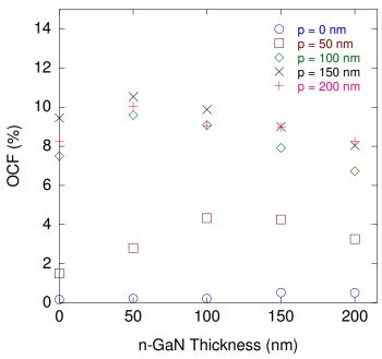
Figure 12 OCF vs n-GaN Thickness for p-GaN = 0, 50, 100, 150, 200nm
