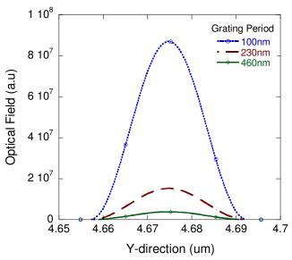
Figure 17 Optical field vs y-direction for mode [9,0]; grating periods 100nm, 230nm, and 460nm
