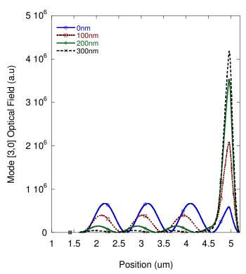
Figure 8 Mode [3,0] optical field vs position for AlGaN thicknesses 0, 100, 200, 300nm
