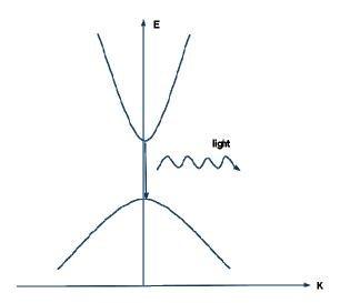
Figure 1 Example of a direct band gap emitting a photon
