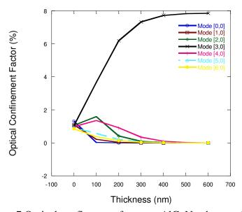
Figure 7 Optical confinement factor vs AlGaN substrate thickness
