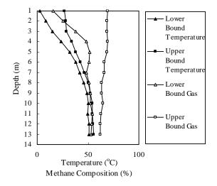
Figure 7. Envelopes for temperature and gas concentration with depth.
