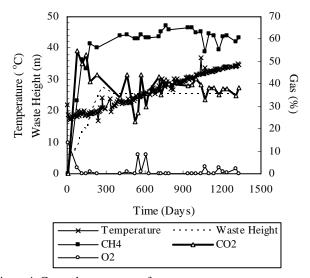
Figure 4. Gas and temperatures for waste.
