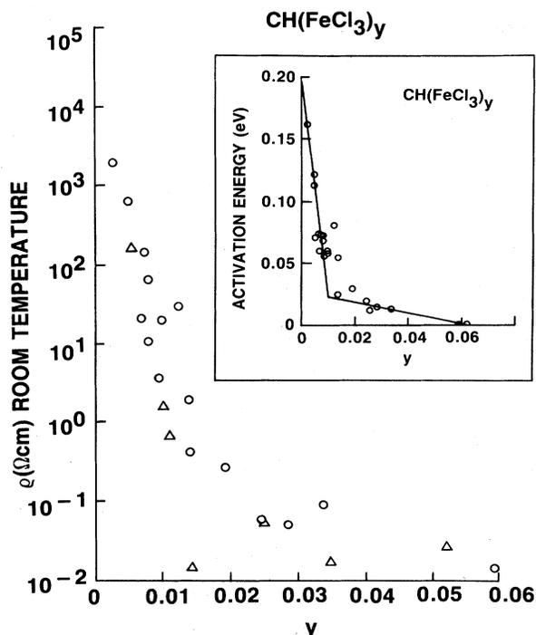
FIG. 3. Room-temperature resistivity of  $\text{CH}(\text{FeCl}_3)_y$  as a function of dopant level  $y$ . Inset shows the activation energy, determined from an Arrhenius plot of the resistivity between 300 and 100 K, as a function of dopant concentration  $y$ .
