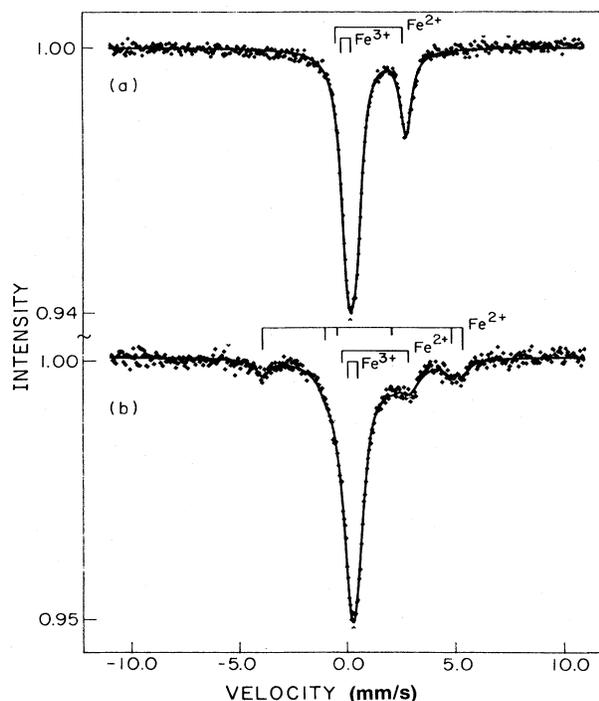
FIG. 1. Mössbauer spectra for CH(FeCl<sub>3</sub>)<sub>0.011</sub> at (a) 40 K and (b) 4.2 K. Parts of the Fe<sup>2+</sup> lines are split magnetically in the 4.2-K spectrum.
