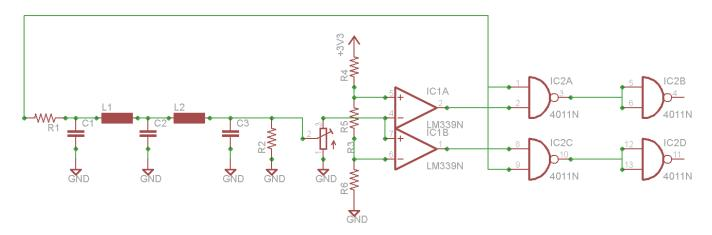
Figure 4.3 Control Circuit Configuration (High Logic): shows the configuration of the logic gates after the comparators
