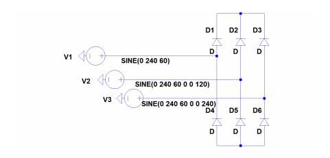
Figure 2.1 Rectifier circuit (discreet component design)
