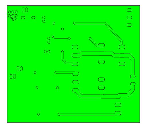
Figure 11.5 bottom level of Diver Circuit (Power Circuit with Gate Driver) circuit PCB layout
