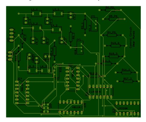
Figure 11.2 Control circuit component layout on PCB
