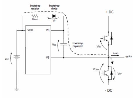
Figure 4.5 Charge Pump Circuit: The component connections made for a single phase on the driver
