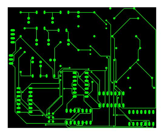
Figure 11.3 top level of control circuit PCB layout
