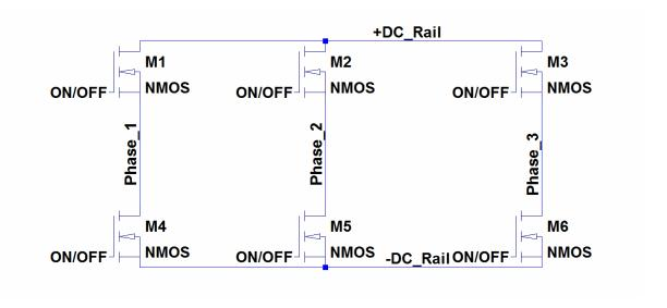
Figure 2.3 H-bridge Configuration: terminals have been labeled to identify phase
