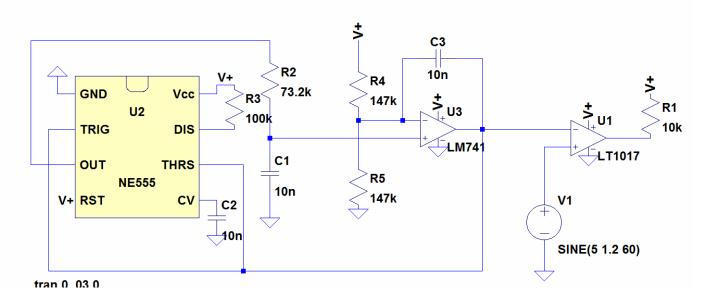
Figure 2.5 PWM Generation Circuit: The circuit consist of a comparator with a triangle wave and a sin wave for inputs, the output of the circuit is PWM.
