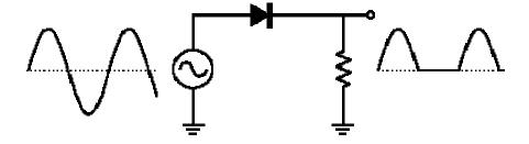
Figure 3.5 Half Wave Rectifier Circuit: Circuit applied to a single phase with a pull down resistor at output (only shows the + portion)
