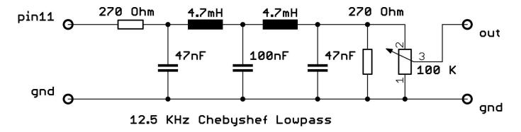
Figure 3.3 Chebyehef Low-Pass Filter: the low pas filter used to go from PWM to a Sin wave it cuts off at 12.5kHz as well as filter out the 32kHz signal used for sampling
