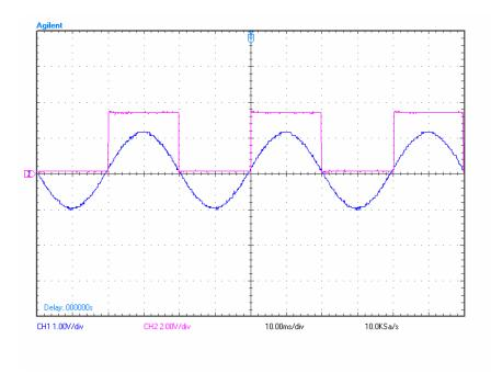
Figure 4.2 Enable Circuit Input/Output: CH1 is the filtered sin wave, CH2 is the enable signal
