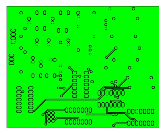
Figure 11.4 bottom level of control circuit PCB layout
