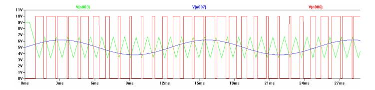
Figure 2.6 PWM Simulation Results: (top) 60Hz sin input (Bottom) 80Hz sin input
