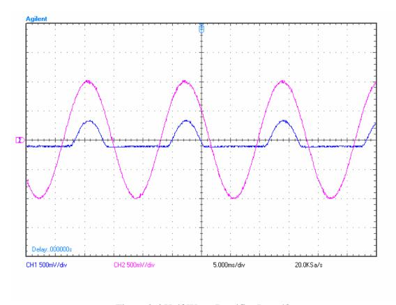
Figure 3.6 Half Wave Rectifier Input/Output: Signals after the half wave rectifier circuit
