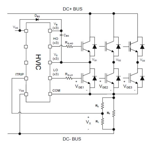
Figure 3.2 Gate Driver IC Typical Application: Shows a basic implementation of the International Rectifier Gate Driver with external BJT switches
