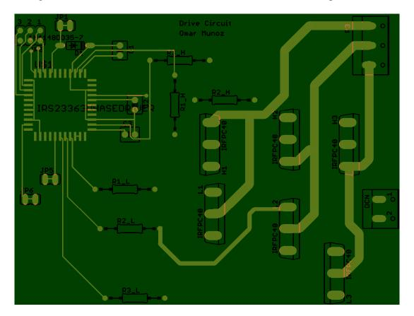
Figure 11.6 Driver Circuit component layout on PCB
