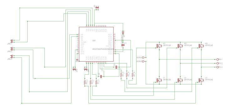
Figure 11.5 Diver Circuit (Power Circuit with Gate Driver) at component level
