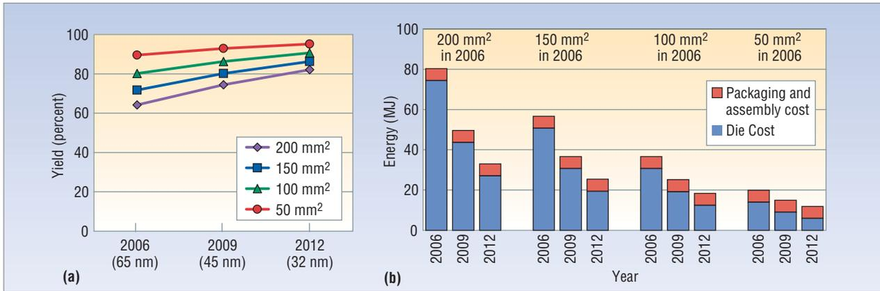
Figure 1. Semiconductor yield and manufacturing energy costs over time. (a) Shrinking the processor increases yield, which (b) decreases manufacturing energy costs over subsequent generations.
