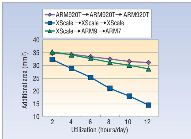
Figure 4. Chip area available for additional circuitry on three processor reuse chains while still maintaining lifetime energy efficiency.
