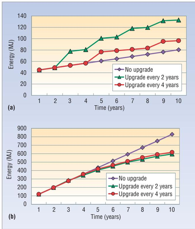
Figure 2. Potential benefits of processor reuse. (a) Upgrading a 1-W processor does not improve the lifetime energy consumption for at least 10 years, making processor reuse an attractive alternative. (b) For processors that use more power—in this case, 20 W—upgrading with newer, more efficient technology makes sense.
