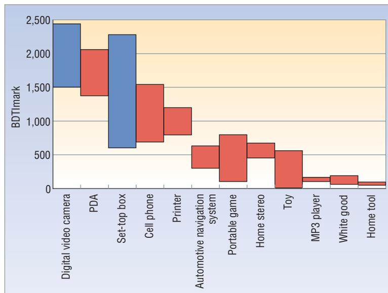
Figure 3. BDTI<sub>mark</sub> performance of various electronic devices. A processor used in a particular device should be capable of handling the processing required by all devices to the right of it.
