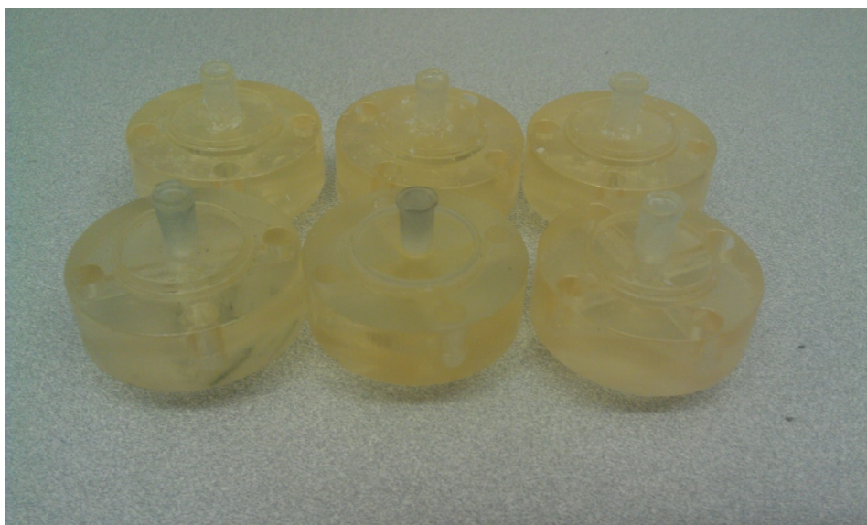
Figure 45. Final Sealant Injectors for the LLNL
