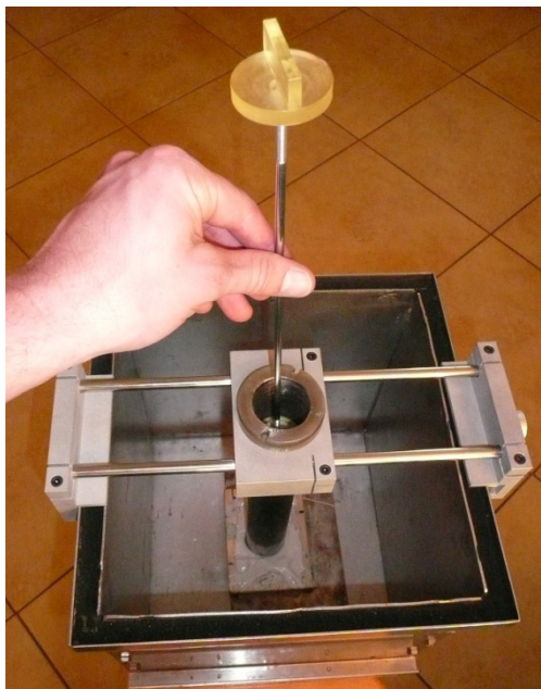
Figure 61. Installing sealant injector assembly
