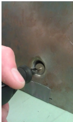
Figure 7. Diamond coated cutting wheel in position
