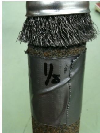
Figure 8. Wire brush in position
