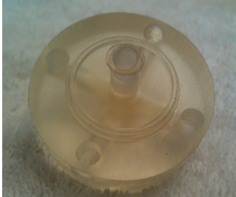
Figure 35. Revision 2 of the Sealant Injector with a Luer Taper
