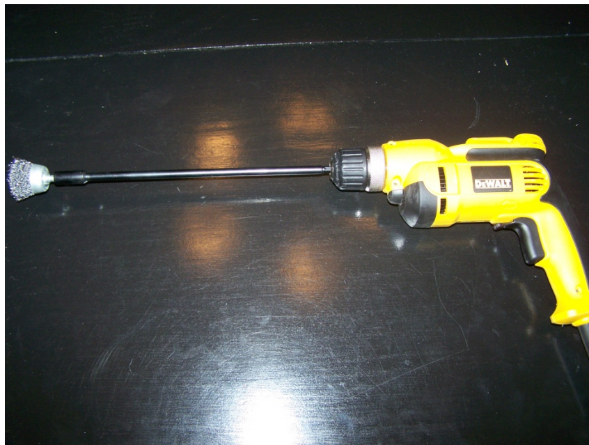
Figure 43. Wire Brush with Extension attached to a Drill
