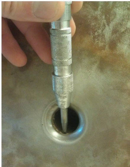
Figure 29. Automatic Center Punch in Position
