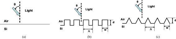
Fig. 1 The schematic diagrams of solar micro-profiles for the simulation. a) flat interface; b) rectangular interface; and c) triangular interface
