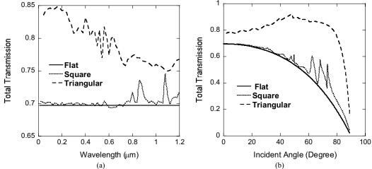
Fig. 2 The transmittance of flat surface (straight line), rectangular profile surface (short dashed line), and triangular profile surface (long dashed line) as function of (a) incident light wavelength and (b) incident light angle.
