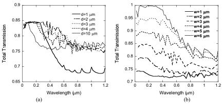
Fig. 3 The transmittance of triangular-profile interface: (a) d=1, 2, 3, 4, and 10  $\mu$ m, w= 3  $\mu$ m, and  $\Lambda$ =6 $\mu$ m and (b) d=3 $\mu$ m, w= 1, 2, 3, 4, 5, and 6  $\mu$ m, and  $\Lambda$ =6 $\mu$ m.
