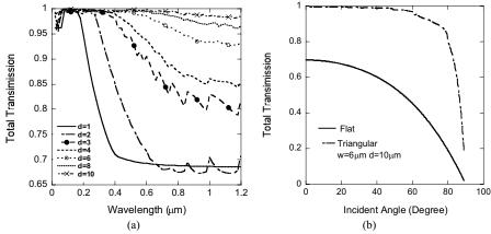
Fig. 4 The transmittance of (a) triangular-profile interface: d=1, 2, 3, 4, 6, 8 and  $10 \mu m$ ,  $w=6 \mu m$ , and  $\Lambda=6\mu m$  and (b) triangular-profile interface  $d=10 \mu m$ ,  $w=6 \mu m$ , and  $\Lambda=6\mu m$  comparison to flat interface
