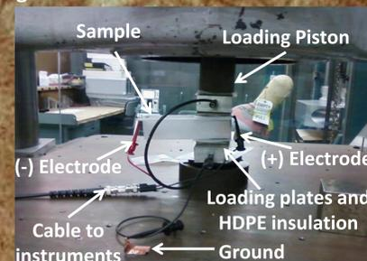
Figure 2. Experiment Setup
