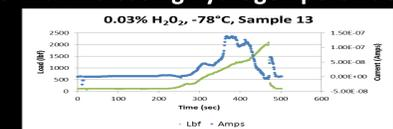
Figure 4. Ideal plot of current vs. load
