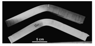
**Figure 4.** The results of the room temperature bend test of the inch thick plate. The top plate was actively cooled and fractured while the bottom plate was conventionally processed. The top surfaces of both plates were completely FSPed to a depth of 7 mm.
