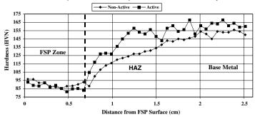
**Figure 2.** The through thickness hardness profile of both the actively cooled plate and conventionally processed plates shows a dramatic increase in hardness upon leaving the FSP zone. The actively cooled plate recovers its hardness over a shorter distance relative to the conventionally processed plate. The dashed line indicates the border between the FSP zone and the HAZ.
