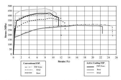
Figure 3. Representative curves of the room temperature tensile tests. Note the large increase in ductility and depressed strength in the FSP zone of both actively cooled and conventionally FSP plates.
