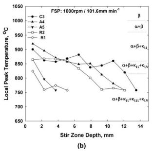
Fig. 8—(a) Transverse view of the SZ, TMAZ, and base metal microstructures for material processed at 1000 rpm and an intermediate traversing rate of 101.6 mm min<sup>-1</sup>. (b) Microstructure-based estimates of local peak temperature as a function of SZ depth for five different downward traverses through the SZ. These data suggest that advancing and retreating sides exhibit similar temperature-depth profiles.
