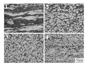
Fig. 5—Higher-magnification micrographs from locations denoted 1 through 4 in Fig. 4(a) for material processed at  $1000~\rm rpm$  and  $50.8~\rm mm~min^{-1}$ .
