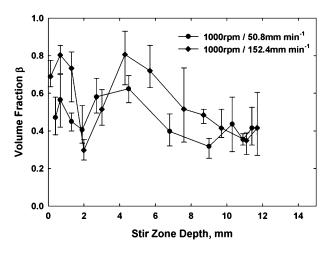
Fig. 6—Volume fraction of  $\beta$ ,  $V_{\beta}$ , as a function of SZ depth for materials processed at 1000 pm and either 50.8 or 152.4 mm min<sup>-1</sup>. Average values of  $V_{\beta}$  as well as the range of values are plotted.
