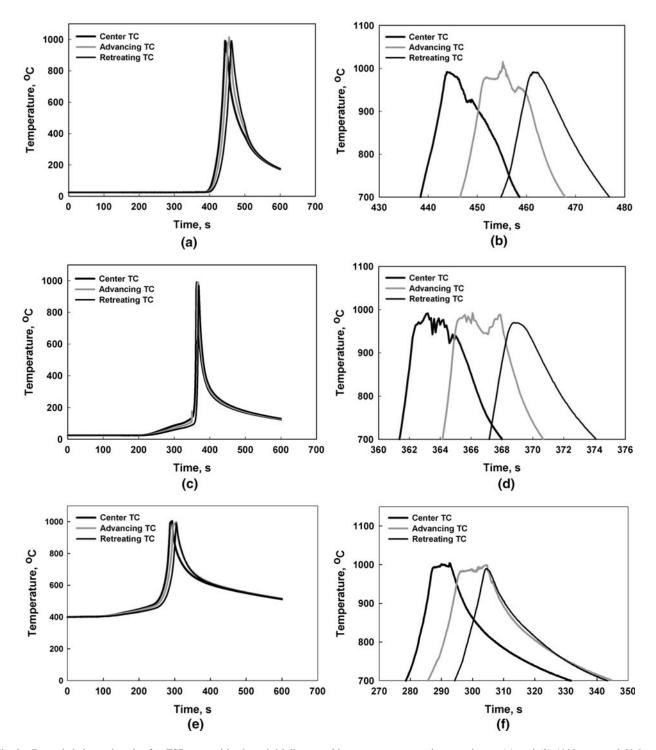
Fig. 2—Recorded thermal cycles for FSP runs with plates initially at ambient temperature and processing at (a) and (b) 1000 rpm and 50.8 mm min<sup>-1</sup> and (c) and (d) 1000 rpm and 152.4 mm min<sup>-1</sup>. (e) and (f) Thermal cycles for material preheated to 400 °C and processed at 1000 rpm and 50.8 mm min<sup>-1</sup>. Complete thermal cycles are presented in (a), (c), and (e), while the portions of the thermal cycles above 700 °C are presented in (b), (d), and (f).
