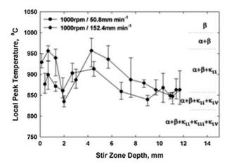
Fig. 7—Corresponding microstructure-based estimates of local peak temperature and range of peak-temperature values for the  $V_{\beta}$  vs depth data of Fig. 6 are shown. These data indicate that the maximum temperature value is at a SZ depth of ~4 mm.
