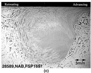
Fig. 4—Transverse cross-sectional views of the SZ, TMAZ, and base metal for NiAl bronze material processed at ambient temperature and (a) 1000 rpm and 50.8 mm min $^{-1}$ , (b) 1000 rpm and 152.4 mm min $^{-1}$ , and (c) after preheating to 400 °C and processing at 1000 rpm and 50.8 mm min $^{-1}$ .
